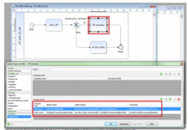
2. On node-leave the set variable is send to the mainprocess with the help of the [WriteBackProcessVariableHandler](#).
