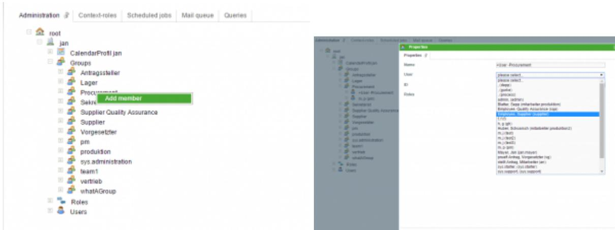
Adding a user is done by right-clicking on the respective group. Subsequently, an existing user must be assigned to the new membership.
