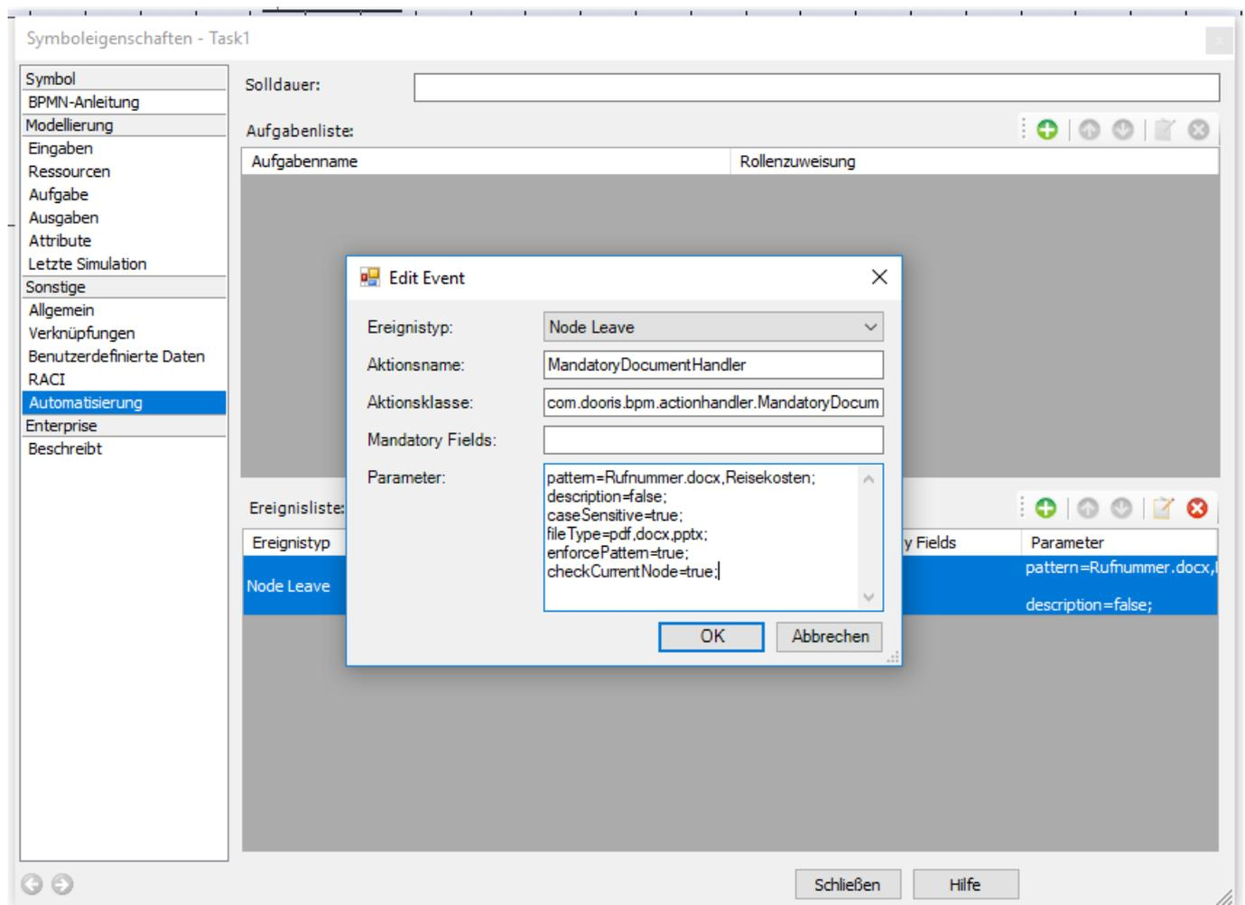
**Attention!** If the check should only determine if a document is attached, the action handler will be executed without the parameter!
